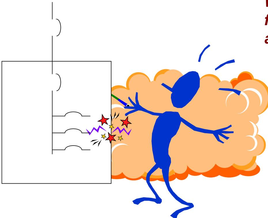
**1. The circuit breaker or fuse clears the circuit to stop the arcing.**
