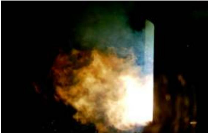
**The amount of energy impressed on a surface, a certain distance from the source, generated during an electrical arc event.**
